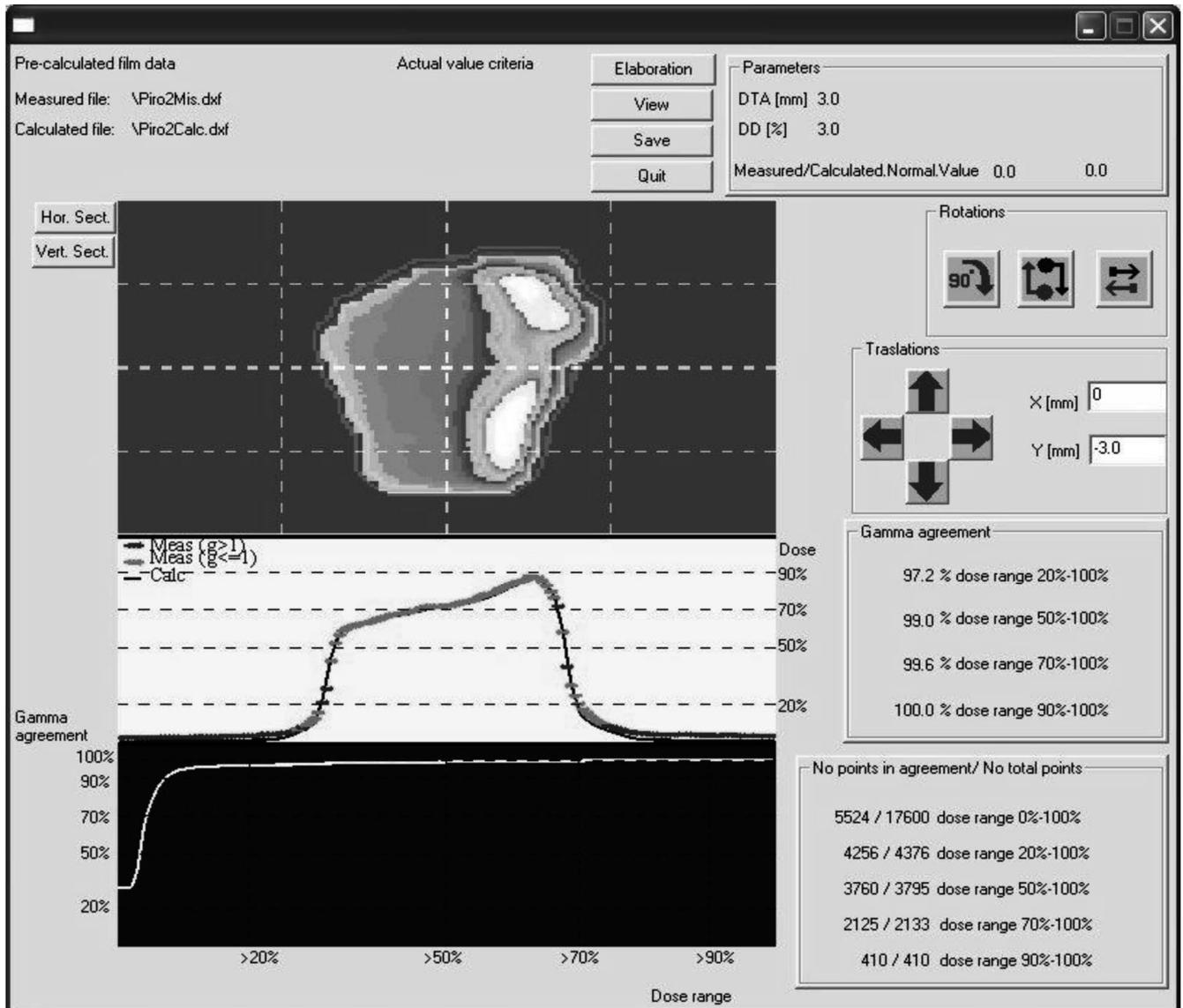
Fig. 1 - Comparison between film and calculated plan. Prostate.
